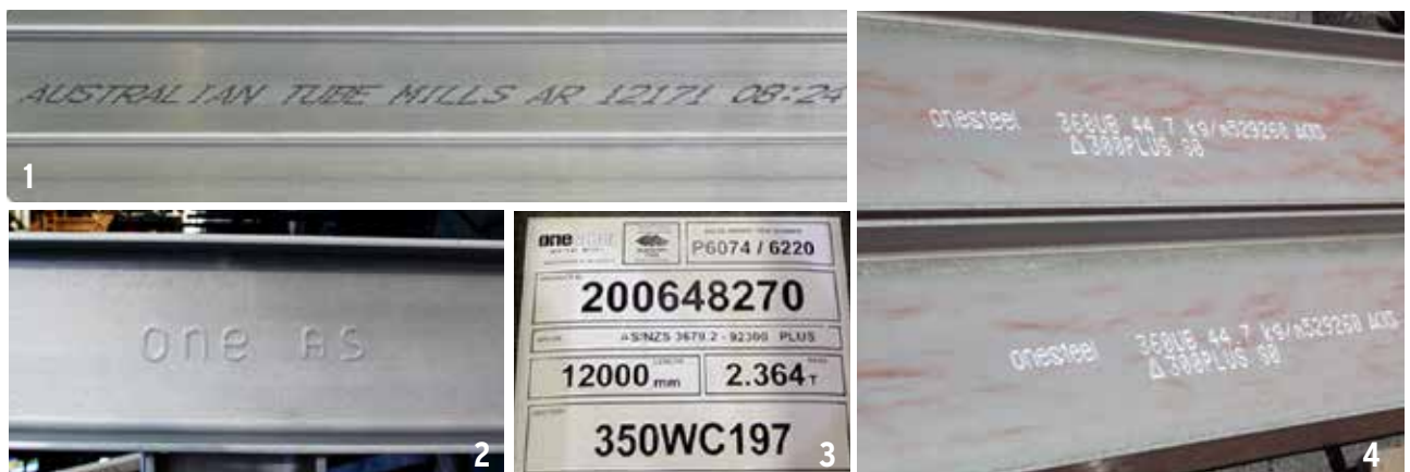
1. AS/NZS 1163 Hollow Sections marking 2. Rolled-in mark on AS/NZS 3679.1 Structural Products 3. AS/NZS 3679.2 Welded Product marking 4. OneSteel stencil marking (not mandatory)
